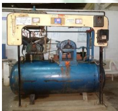
Two Stage Single Acting Reciprocating Air Compressor Test Rig
