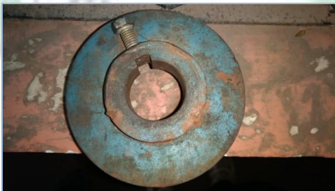
Fig. Motor pulley before maintenance
